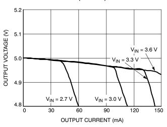
Figure 4. Output Voltage vs. Input Voltage
