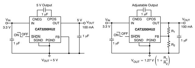
**Figure 1. Typical Application Circuits**
