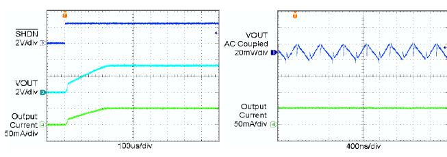
Figure 18. Power Up Waveform (I<sub>OUT</sub> = 50 mA)
