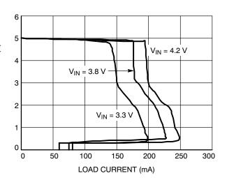
Figure 13. Foldback Current Limit
