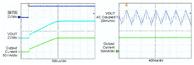
Figure 10. Power Up Waveform (I<sub>OUT</sub> = 100 mA)
