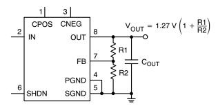
Figure 20. Programming the Adjustable Output
