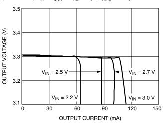
Figure 14. Output Voltage vs. Input Voltage
